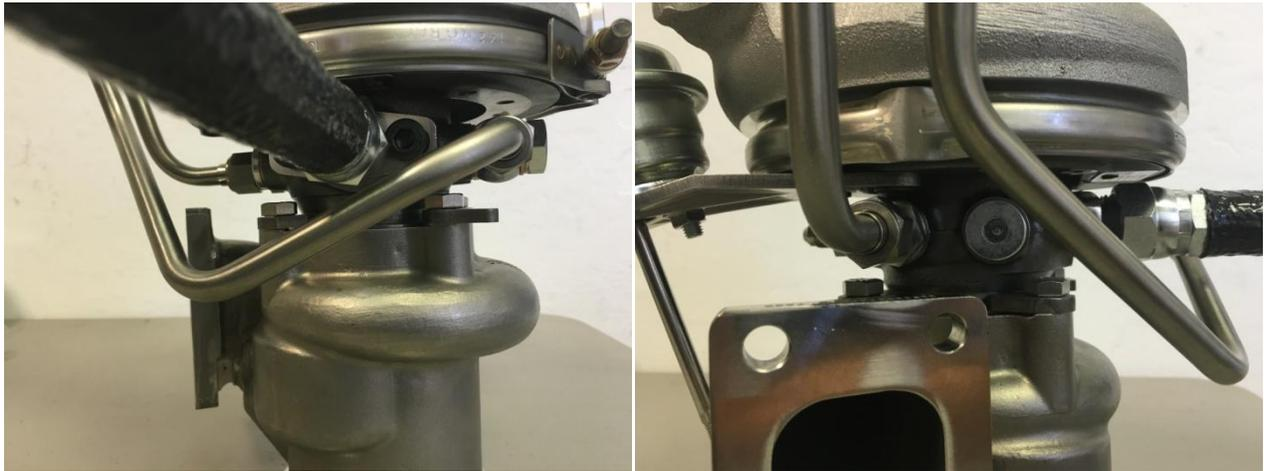
Use the provided short silicone hoses and hose clamps to attach the water lines to the engine as shown. If you have deleted the front water neck, attach the hose to the throttle body hose or to the factory oil warmer. If you have a 94-97 engine, your water ports are 5/16". The 3/8" hoses should tighten down onto your smaller fittings, but if you want smaller silicone hoses, contact us.
