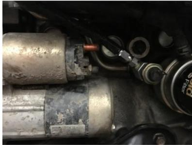
Use teflon tape or paste on the -4AN to 1/8" NPT adapter, then thread the NPT side into the side port of the adapter. Tighten until finger tight, then add 2 turns with a wrench. Use teflon tape or paste on the OEM pressure sensor and install it in the end of the oil feed adapter. Tighten until hand tight, then add 2 turns.
